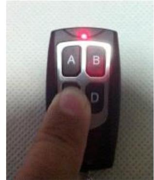
When pressing a button hold the button down for about half a second. A button press which is too short will be ignored and a button press which is too long may cause an undesired mode change. A bit of experimentation will allow you to get to know the required button press durations.
